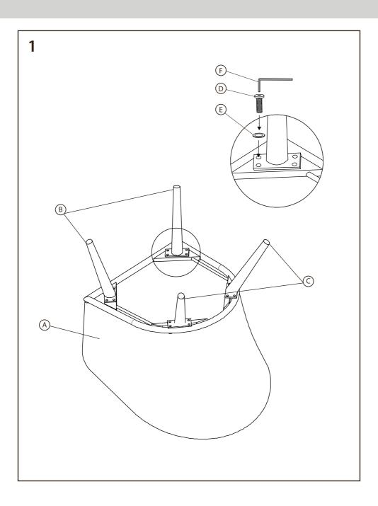
2 Assemble all parts loosely and when all components are in place tighten fixings to secure
